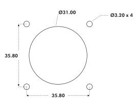
The joystick flange is mounted beneath the panel and the base of the gaiter must be brought through the panel cut-out and held in place with the circular bezel. For panel thicknesses of 3mm, M3 x 16 countersunk machine screws are recommended.
