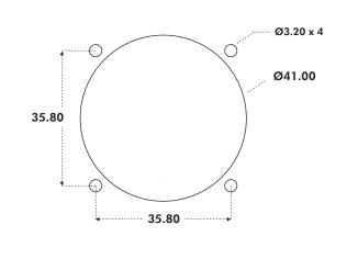
The joystick is dropped into the panel cut-out. For panel thickness of <3mm, M3 x 16 countersunk machine screws are recommended.
